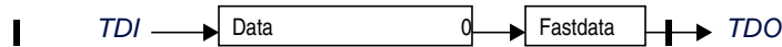
Figure 11.16 TDI to TDO Path When in Shift-DR State and FASTDATA Instruction is Selected
